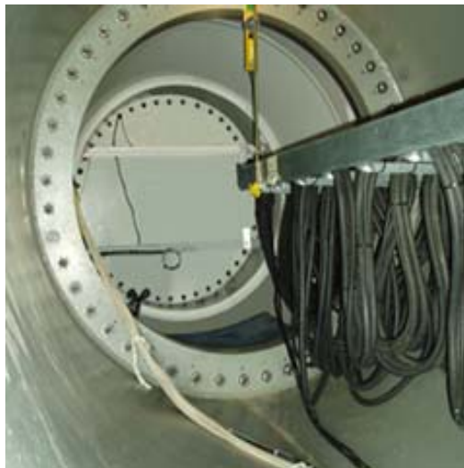
Figure 4-12. Droop loops were hung from the cable tray to take up the slack.
