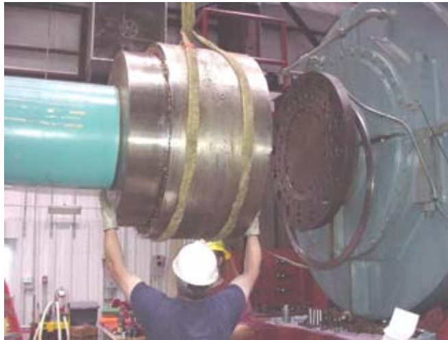
Figure 4-11. The coupling was installed after the generator and dynamometer shafts were aligned.
