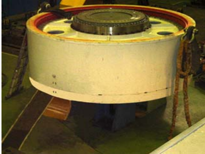
Figure 4-6. A final acceptance test was performed at the generator manufacturing facility, but the generator was too large for the facility's dynamometer.
