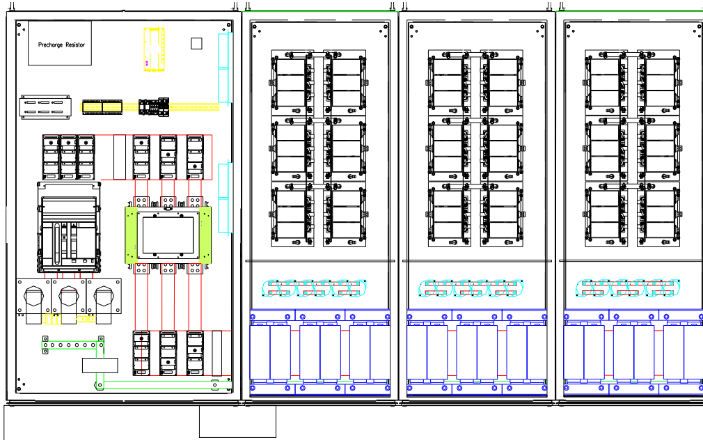
Figure 3-2. The power electronics system was made from three 500-kW modules.
