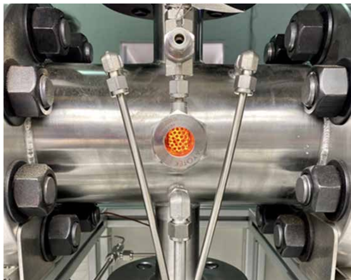
To capture natural gas instead of burning it, the MAC team uses a microwave reactor with an electric-based process to convert the methane into a higher-value chemical commonly used in plastics manufacturing. Photo from MAC, NETL
